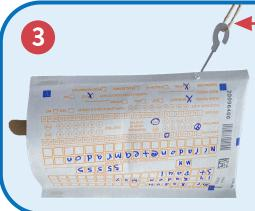
Hang the test kit up by its hook. Keep up 3 – 7 days.
